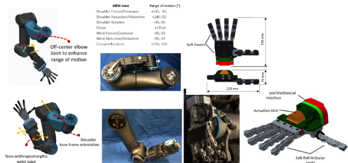
Figure 3: The robotic manipulator arm and the end-effector hand – design and prototype.
